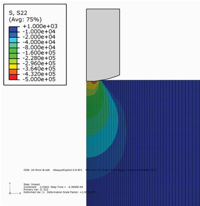
Fig. 2. Typical distribution of vertical normal stresses in concrete during the rebound hammer impact obtained by means of FE analysis. Stresses at the beginning of the rebound
