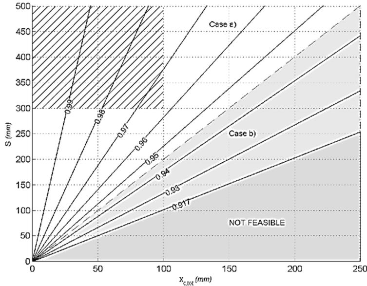
Fig. 4. Theoretical values of  $k_v$  for different values of  $S$  and  $x_{c,tot}$
